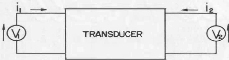
Figure 1. Functional diagram of a four-terminal transducer.
